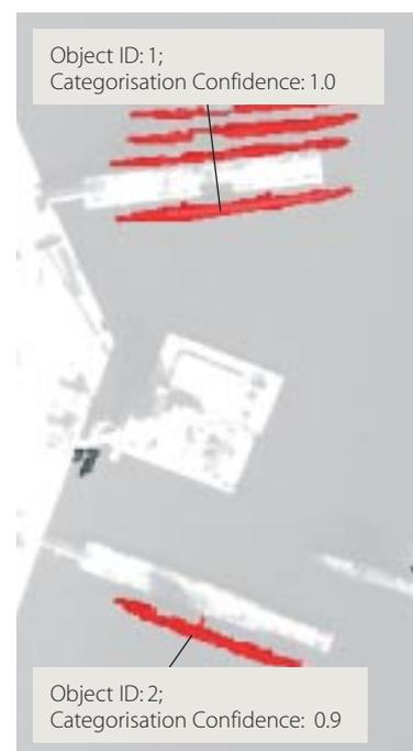
Within the panchromatic satellite imagery (QuickBird) five vessels are detected as image objects and categorized as diesel submarines (red objects). The result is ready to be used in a geodatabase to monitor statistical movements in the area and to detect anomalies.
