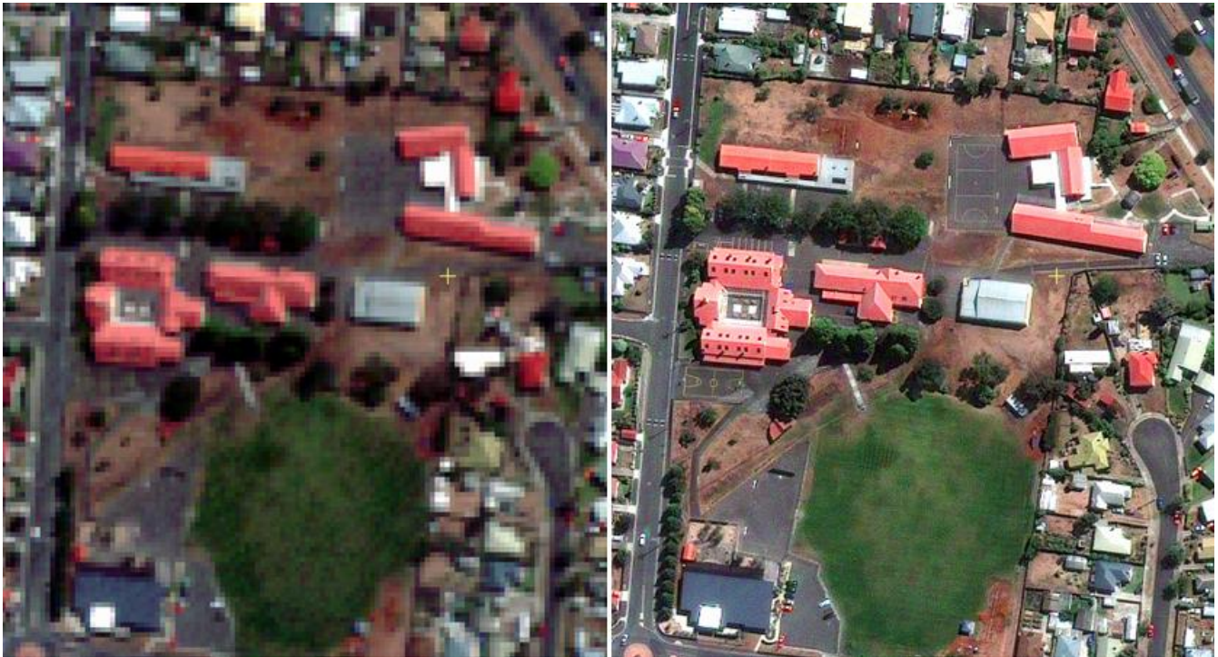
Figure: Comparison of raw resolution multispectral image (left) and pansharpened image (right)
