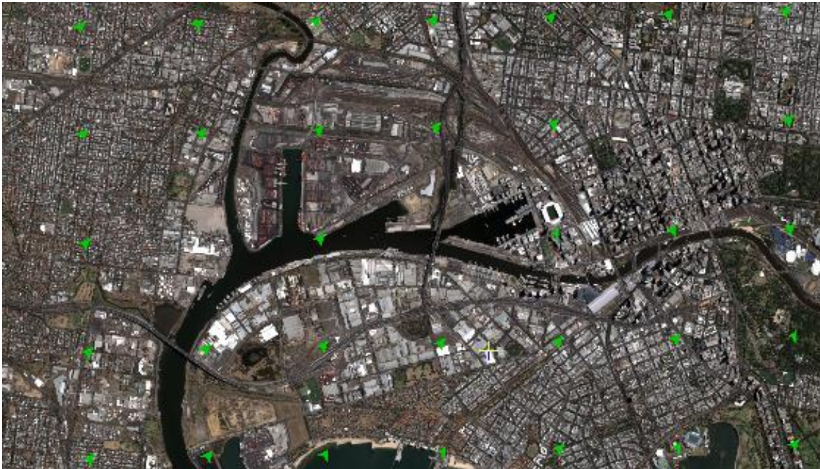
Figure: Example of sub-pixel GCPs collected in an even grid layout throughout the input Pleiades image
