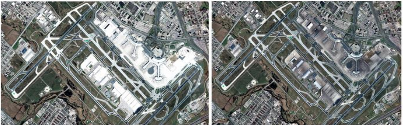
Figure: Over-exposed airport before and after correction applied
